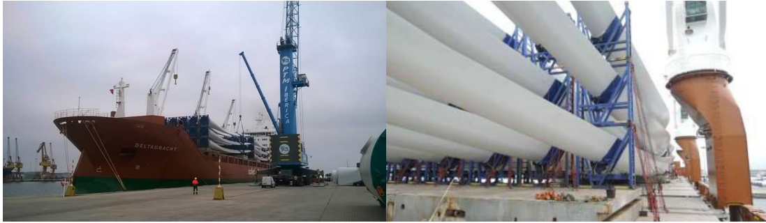
LEFT AND RIGHT: blade and turbine components on board the ship en-route to site.
